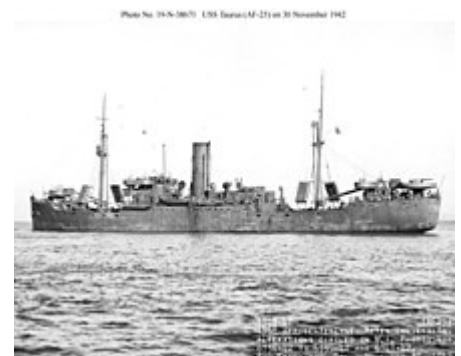
USS Taurus , which was built as San Benito in 1921, may have been the world's first turbo-electric merchant ship
